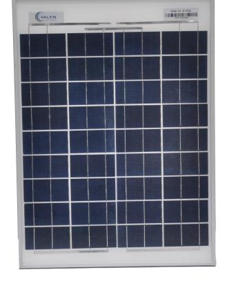
• A corrosion-resistant module frame made of anodized aluminium alloy provides high mechanical strength to resist wind and hail storms. The frame has mounting holes on the side rails to bind the module to other supporting structures ensuring ease of installation.
