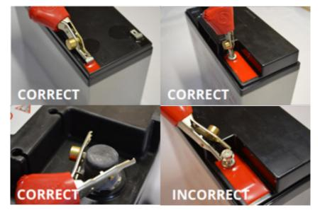
WARNING! The IBT Chrome will produce accurate, consistent Ah readings only when connected directly to clean battery terminals. Low, erratic Ah readings will be obtained when connecte to high resistance bolts or cables attached to the battery posts.
